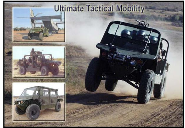
**Description:** The existing ITVs are designed to be internally transportable in a CH53E helicopter. Its mobility exceeds the HMMWV and is capable of serving as a heavy machine gun platform. The vehicle crew consists of the driver plus three Marines. It is capable of supporting the C2 systems organic to an infantry company.
