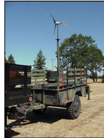
Tactical Alternating Current System (TACS)
