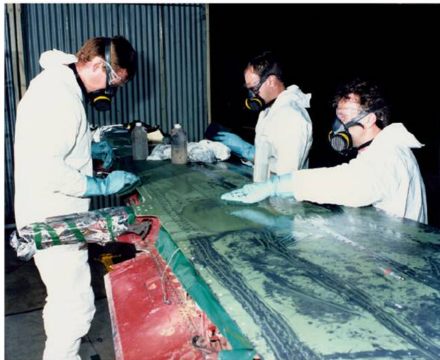
RAAF Maintenance workers cleaning residual sealant from the wing of an F111 after completion of resealing and replacement of the top of the wing.
