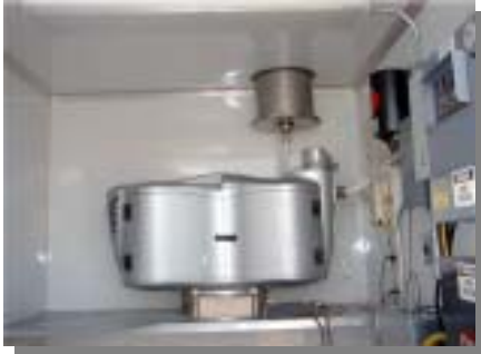
Portal Shield Bio Detector
