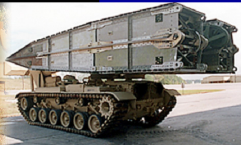
M60 Armored Vehicle Bridge Launcher
