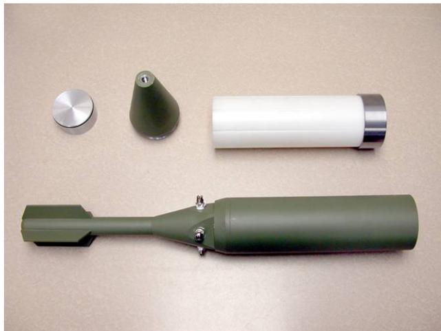
Static Test Hardware (81mm mortar)
