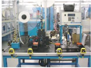
The disc insulator is manually assembled to the terminal plate assembly, and the anode lead is then welded to the center-pin of the terminal plate.
