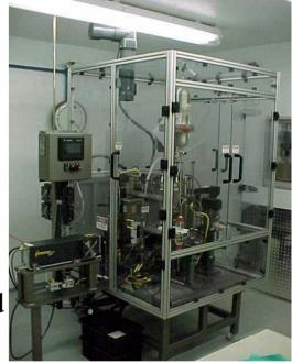
The fill level of Thionyl Chloride in the ampule is monitored on an hourly basis using in-process statistical process control (SPC) to verify the accuracy of the fill pump.
