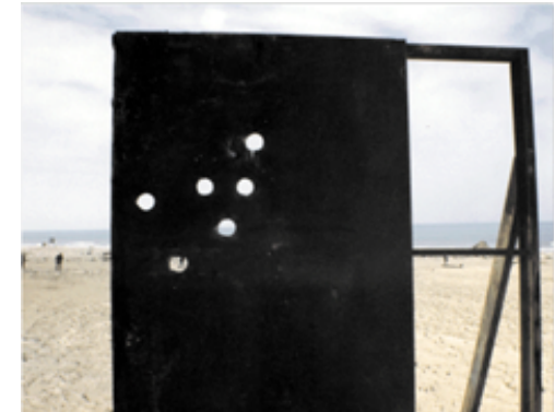
PENETRATION OF 10 mm RHA TARGET BY SUBMUNITIONS
