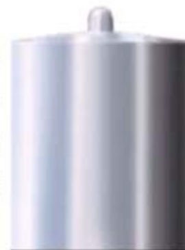
Projectile #2 6.35 mm, 1.6 kg
