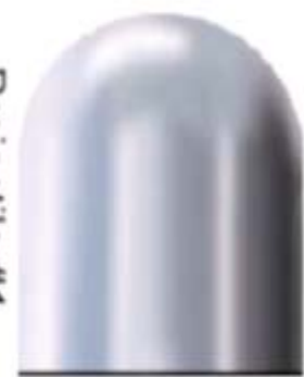
Projectile #1 30.05 mm, 1.2 kg
