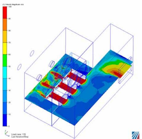
AirePod™ was designed using Computational Fluid Dynamics (CFD) to maximize filter flow uniformity and minimize static pressure losses.
