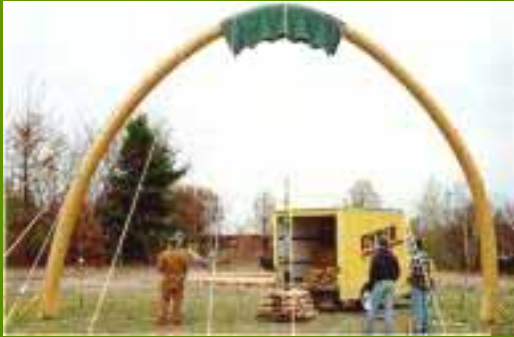
30 foot span, 12" dia, 65 psi
