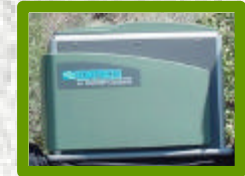
Battery Charging Fuel Cell with Methanol Steam Reforming Unit
