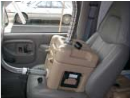
Dry Filter Unit
